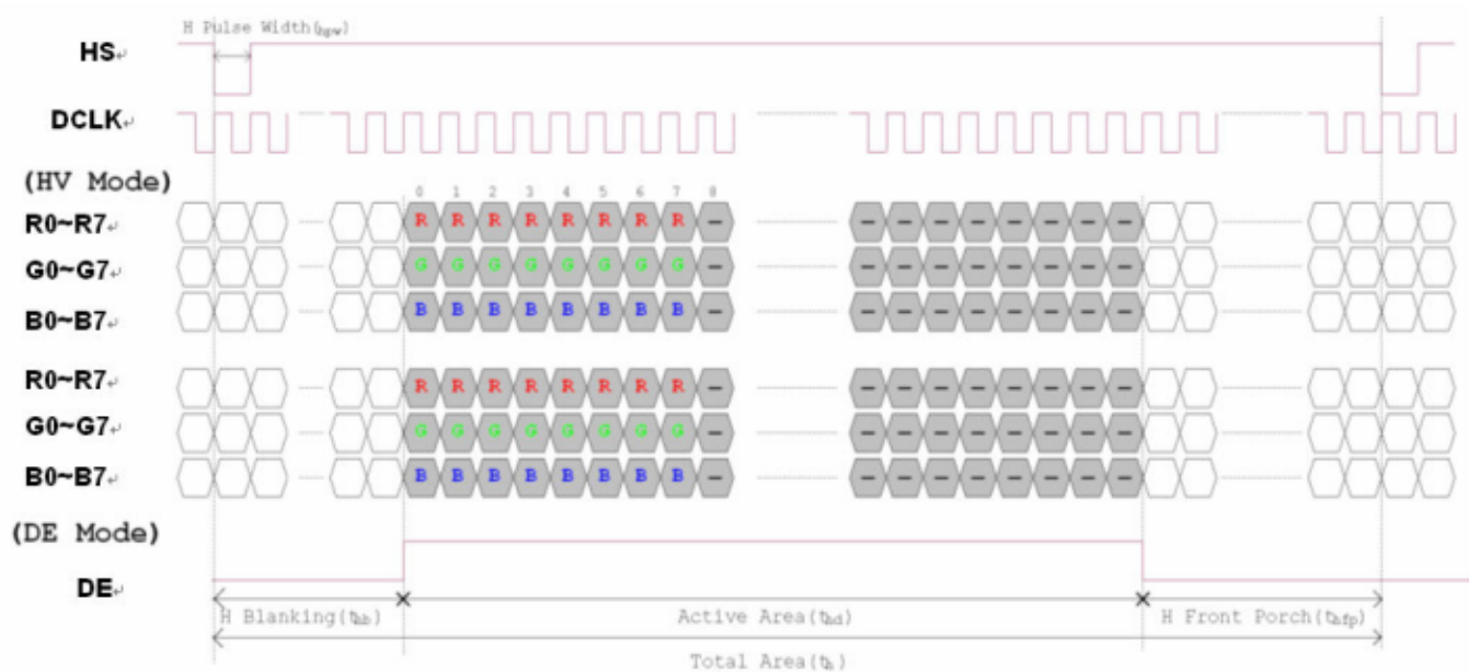
Figure 3. 1 Horizontal input timing diagram.
