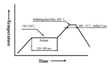
Be careful because damages always caused during soldering. Please note that stress to the leads and expose bulb should be avoided during soldering particularly when heated. When soldering, leave certain distance from soldering joint to base, the distance is determined by different soldering techniques.
