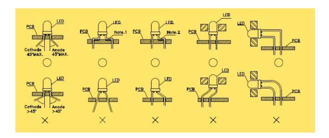
LED flat or make AI, suggest using  $\Phi$  4,  $\Phi$  5 LED chips, to avoid LED chips cracking caused by outside force, and please note dynamics for AI.
